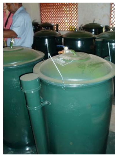
Small biogas units process 0.5-2 kg of kitchen waste daily and cost under €45
